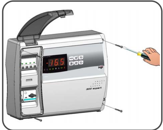
Fig.16: Tighten the front panel using the 4 screws, making sure the O-rings on the head of each screw are used. Reposition screw cover on the right-hand side.
