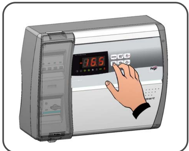
Fig.17: Power up the panel and carry out thorough reading/programming of all the parameters.
