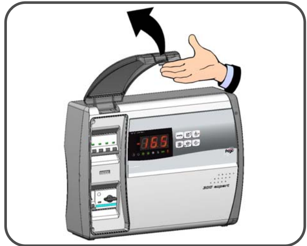
Fig. 1: Pull up transparent cover protecting the general magnetothermic circuit breaker.
